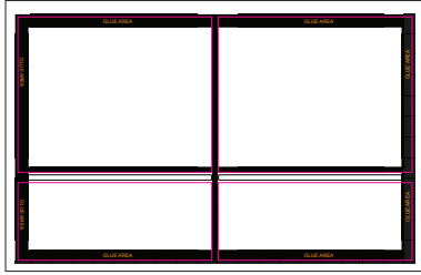
Product No. YD-042 Name: Zip Strip Pocket Folder Sheet size: 19.25" x 12" Size Specs: 9" x 12" with 2-4" Pockets
